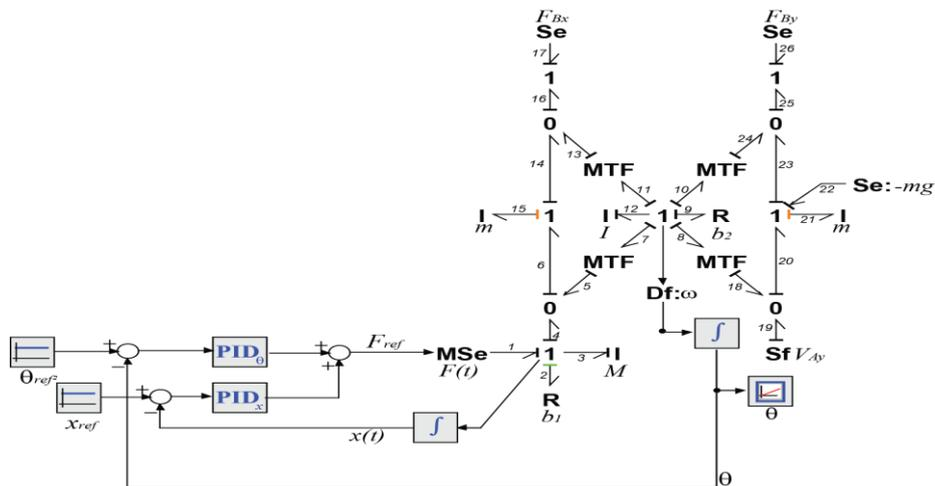
Fig.4 Control structure of PID.
