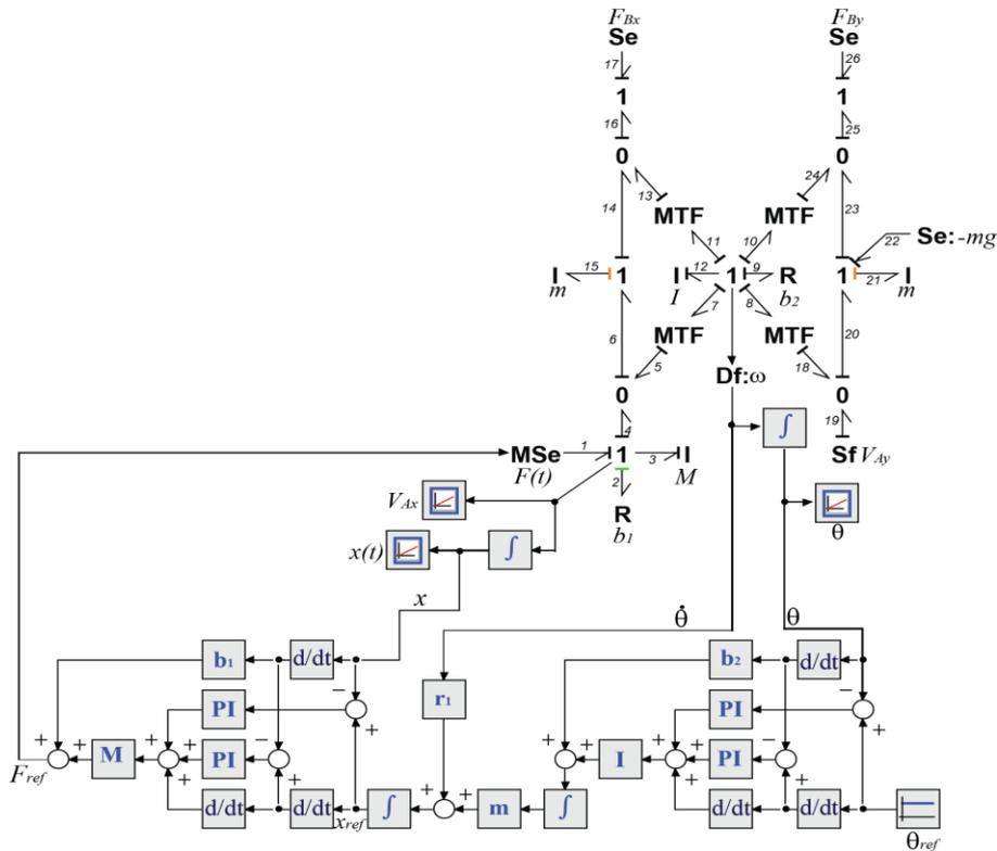
Fig.5 Control structure of IBG.
