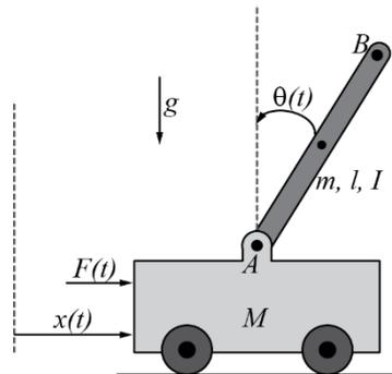
**Fig.2** Schematic representation of an inverted pendulum on a cart.
